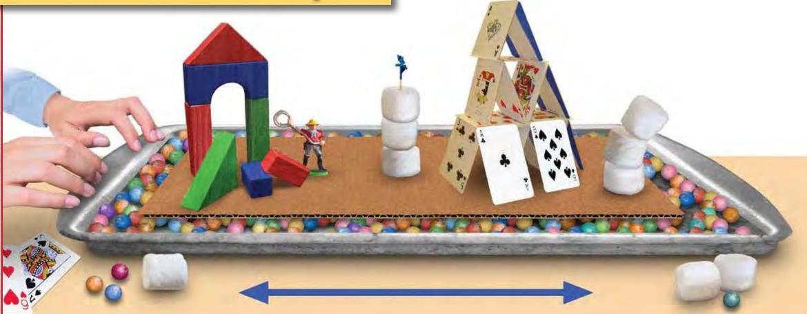
How do you study something that you can't predict? Scientists who study earthquakes and engineers who design earthquake-resistant structures use models. They create "model" earthquakes by using a device called a shake plate. The shake plate simulates the multi-directional movement the Earth experiences during a quake.
