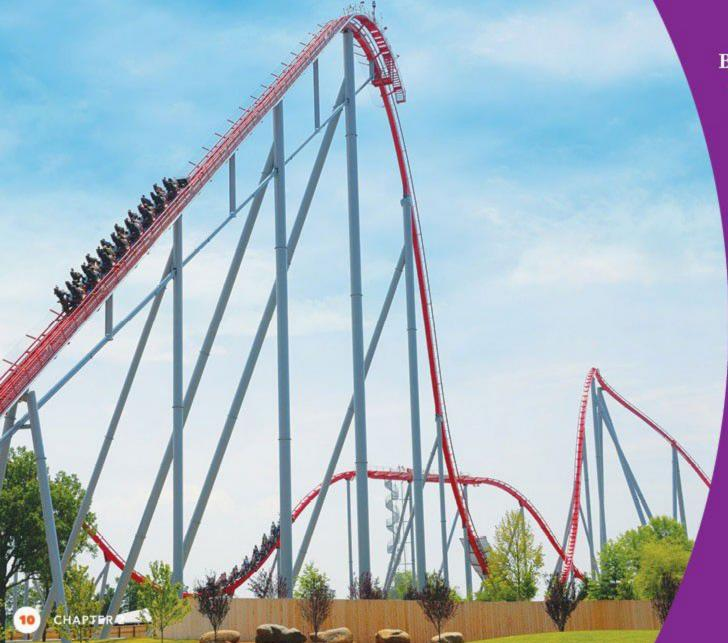
By starting high, the car has the energy it needs to move. This is called potential energy.
